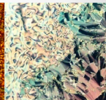
IV, 1C, 300 °C, 200x, Schlieren and focal conic texture
